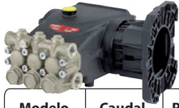
EVOLUTION 3 CULATA DE NICKEL (264x261x117mm | 10Kg | eje Ø25,4mm | SAE 15W40)
